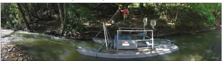
Rotary screw trap in Alameda Creek for trapping fish. Photo: SFPUC
